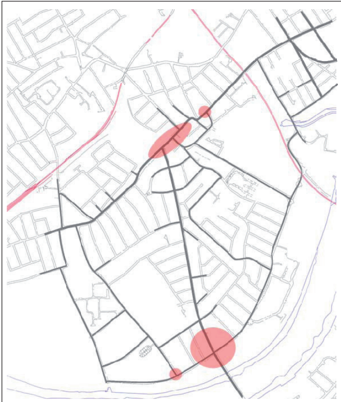
Figure 4.15: Existing stress points on the highway network (size of circle indicates the degree of congestion)
